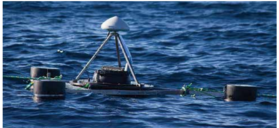
GPS buoy deployed over the Bass Strait moored oceanographic sensors in order to derive an absolute datum for the derived sea level time series. For scale, the white antenna is approximately 0.5 m from the water surface.
