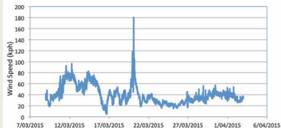
Wind speed measured by the IMOS weather station at Lizard Island during Cyclone Nathan .
