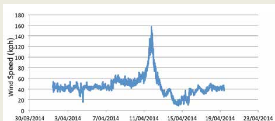
Wind speed measured by the IMOS weather station at Lizard Island during Cyclone Ita .
